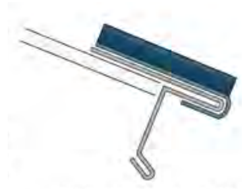
Installation of panel over T-Drip
